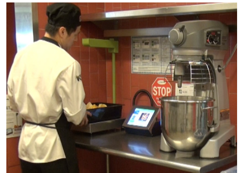
LeanPath system weighs and photographs wasted items for analysis.
